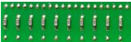
Figure 2: Test vehicle sequentially populated with 0603 capacitors
