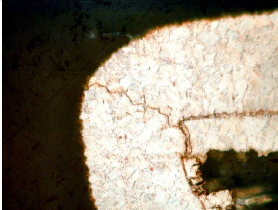
Figure 12 - Corner Crack at a 45° angle.
