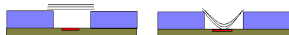
Figure 5. Schematic of the two possible states of a carbon nanotube based memory cell (NRAM).
