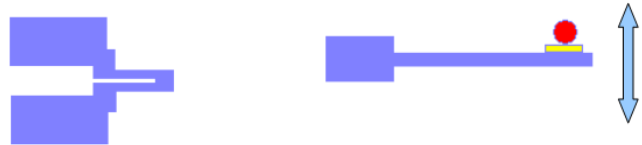
Figure 4. Schematic of a NEMS single molecule detector. Plan view is in the left, side view is on the right
