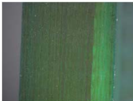
Figure 22: Delamination observed in cross-section of a test coupon subjected to MSL1 exposure (85°C/85RH) and subjected to 3 reflows at a peak temperature of 260°C
