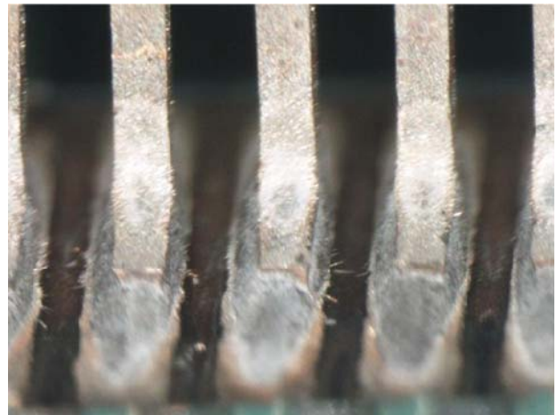
Figure 9. QFP Sample after Completing Etching Process
