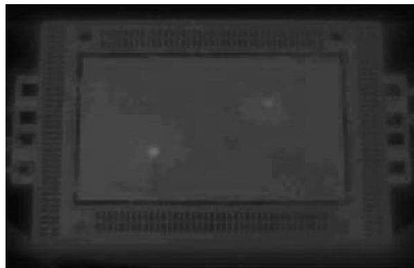
Figure 3. Two imbedded transistor die in an IC/DT® prototype with maximum junction temperatures of 32°C.
