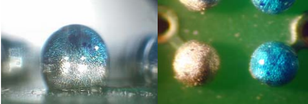
Picture 3: Left image shows an example of a satisfactory dipping process prior to placement using a material coloured blue to aid automatic optical inspection. Right image shows how the solder balls look with, and without, flux coating. This difference may have been caused by variations in the placement height, the flux height or co-planarity issues within the package.
