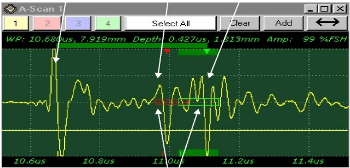
Figure 9 Example of an Acoustic Transducer Response with response gates at special package interfaces of interest
